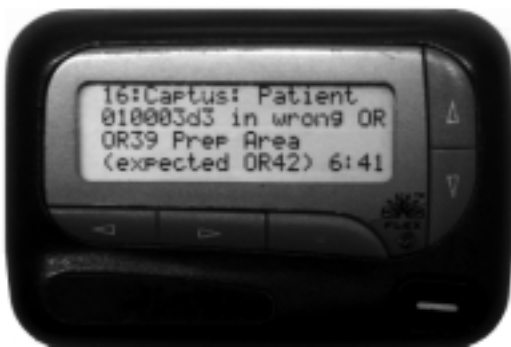
Figure 4. Panel A shows an example of a series of alerts generated by the process monitoring software. The process monitoring software interface is available as a Web page from any personal computer running an Internet browser from inside the hospital firewall. Note that multiple types of process exceptions are detected and generate alerts. Panel B shows an example of a wrong-location alert that appears on the screen of a process manager's pager. In the test setting, the system was configured to pass only the indoor positioning system tag serial number via the paging system to assure compliance with the Health Insurance Portability and Accountability Act of 1996.
